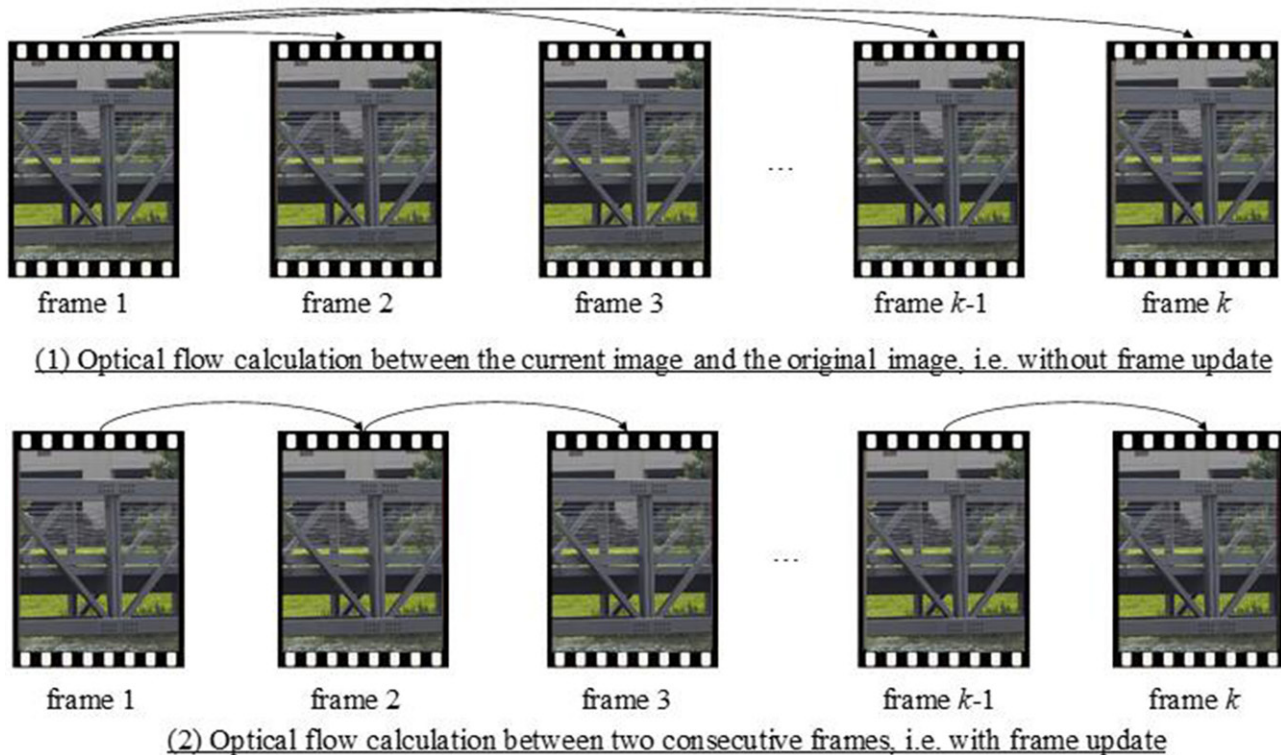
Figure 7. Two different strategies to process image sequences and get displacement time histories.
