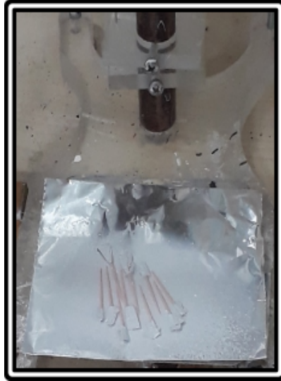
Figure 3.12. Coating process of Gutta-Percha with Nanofiber mats via Electrospinning device
