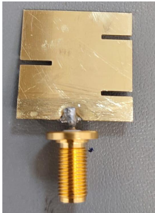
Figure 5. 2 Radiating element is connected to SMA connector
