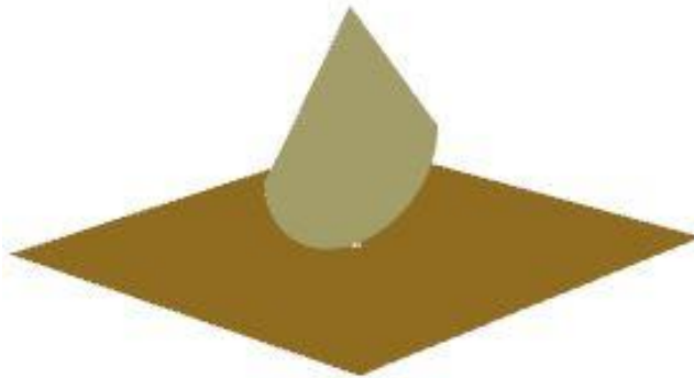
Figure 2. 5 Planar inverted cone antenna
