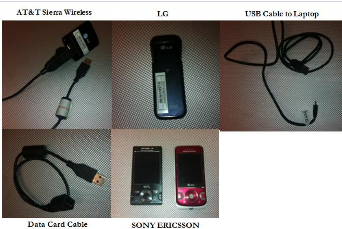
Figure 5.1 Equipment for Drive Test
