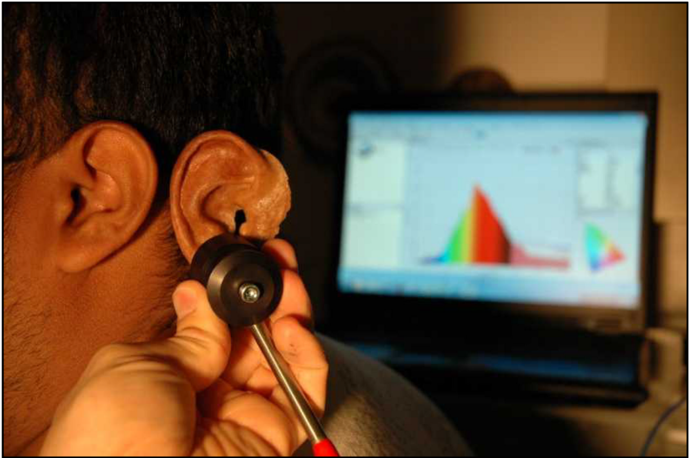
Figure 1. Diffuse reflection spectroscopy measurement of auricular prosthesis adjacent to patient's ear.
