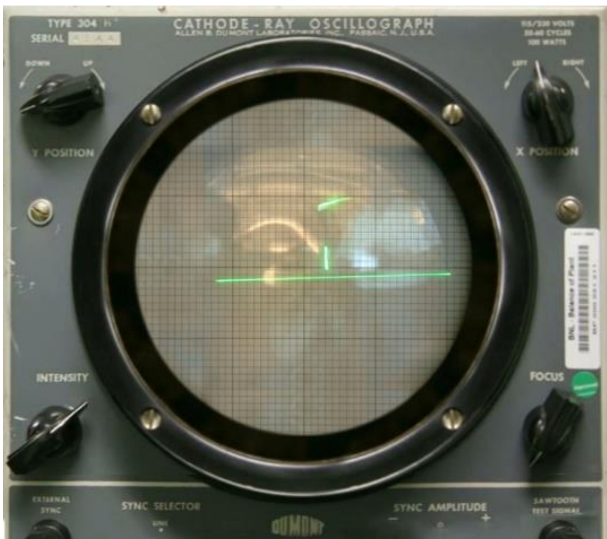
Image 1.1: Tennis for Two computer game on a DuMont Lab Oscilloscope. Source: Brookhaven National Laboratory (BNL), image by Pietro Dipalma.
