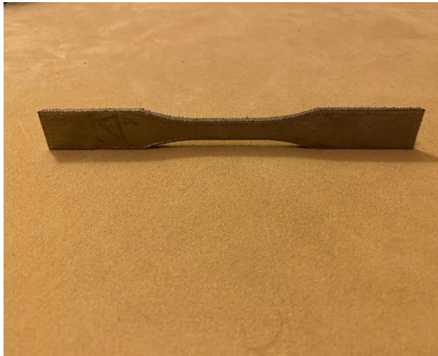
Figure 3.6: Sample Surface Roughness after Manufacturing
