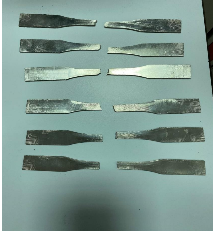
Figure 4.20: Fractured Specimens After Six Tensile Tests
