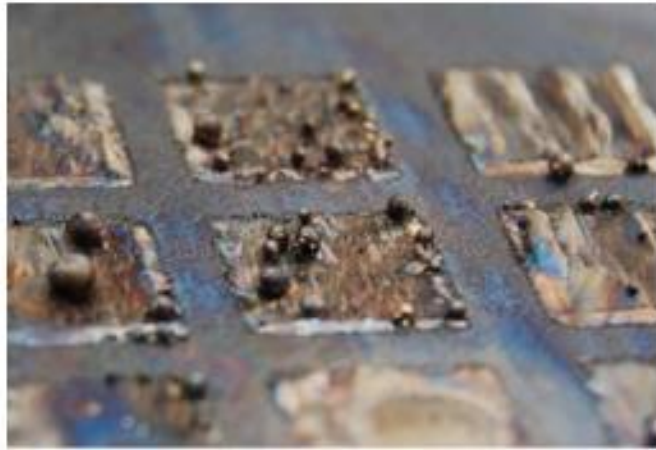
Figure 2.4: Melt ball formation [21]
